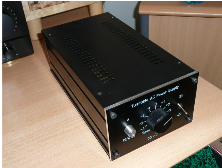
Photo 1: A Power Sinus Generator for a Turntable Synchronous AC Motor
